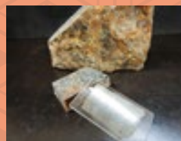
岩石の研磨薄片:厚さ30 \mu m
